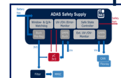
1st Supply for Radar SPT9 DCDC + safety
